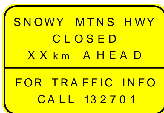
Figure 2 - Advance road closure sign (G9-325-1)
