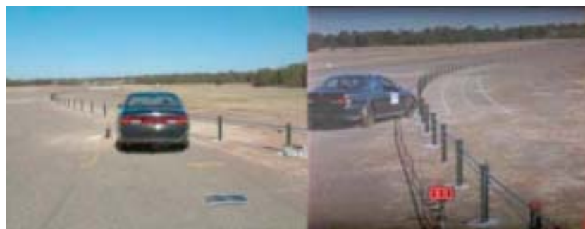
Figure 1 – Test vehicle positioned at an impact angle of 25° to the convex side of the wire rope safety barrier
