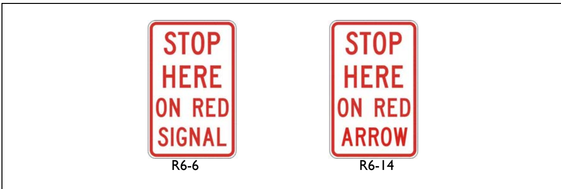
Figure 10.10 STOP HERE ON RED SIGNAL sign
